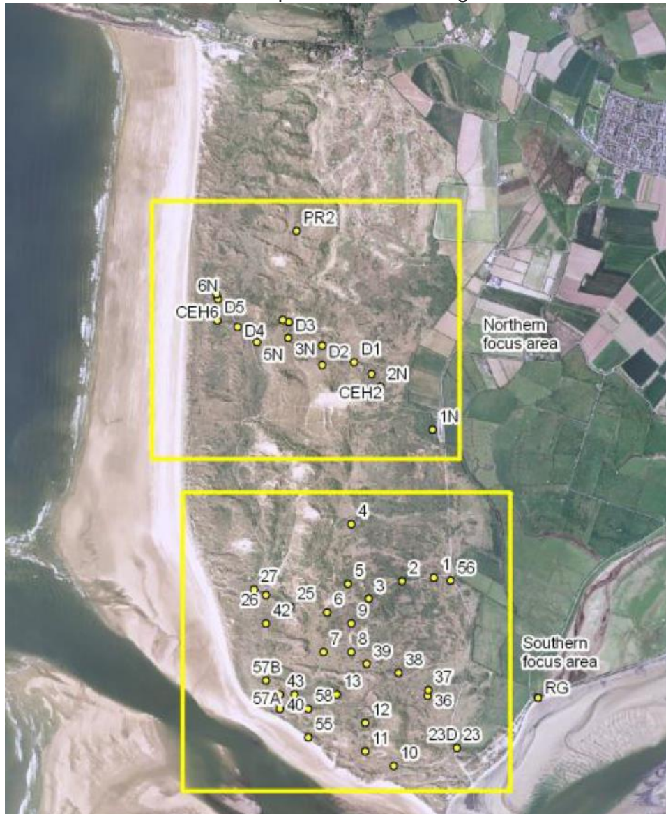
Figure 6 Dipwell monitoring network at Braunton Burrows. Both historic and current monitoring points are shown. (Figure from Report NECR153)
