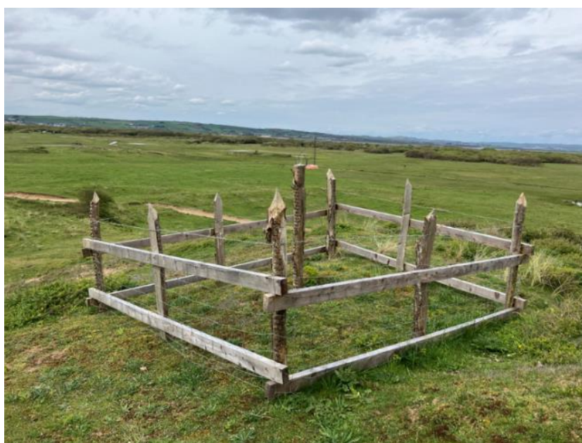
Figure 2: Fenced enclosure with central post supporting ALPHA samplers
