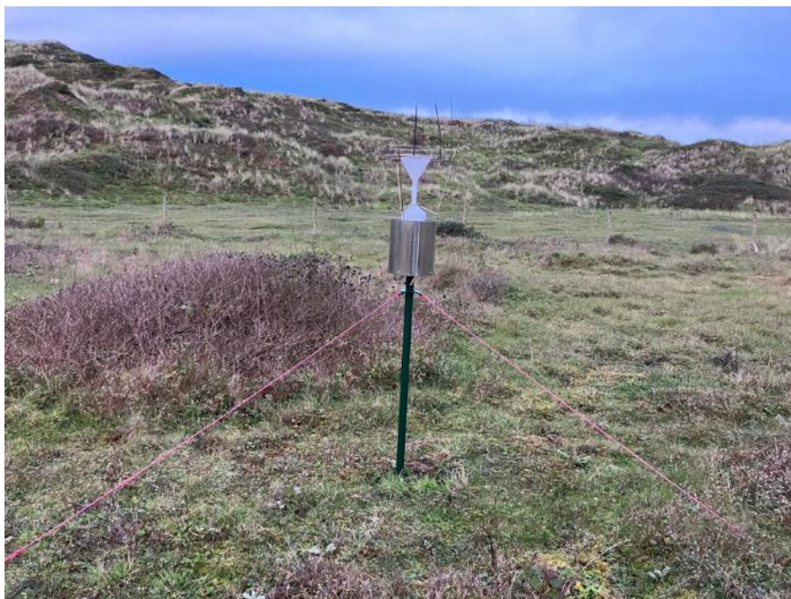
Figure 4: Rainwater collector used for measuring wet deposition of atmospheric Nitrogen contributing to UK Precipitation Network (UK PrecipNet)
