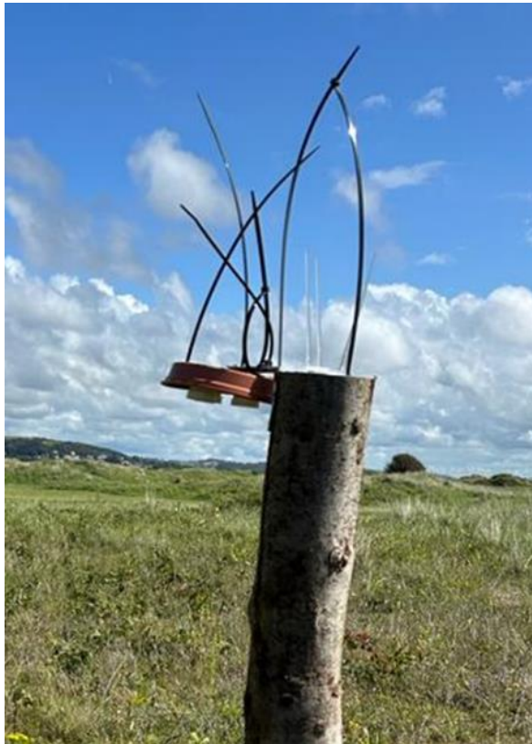
Figure 3: Close-up view of alpha samplers used for measuring dry deposition of atmospheric ammonia.
